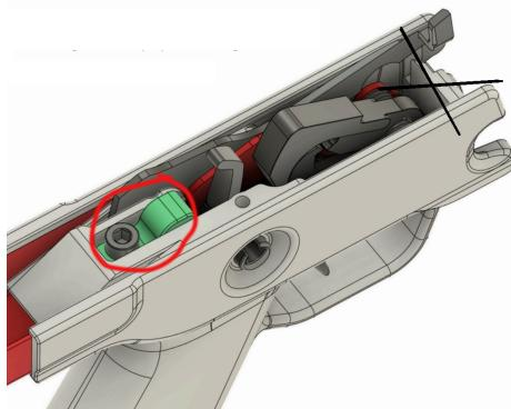
Carefully pry out the cam insert with a small flathead screwdriver
