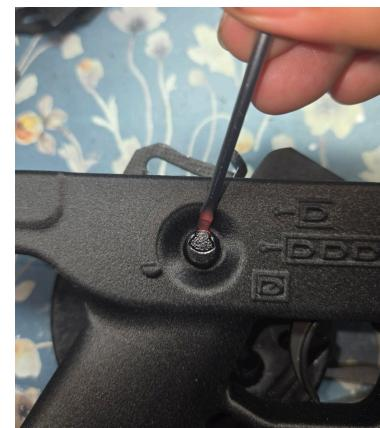
Cock the hammer, insert the flat end of a zip tie between the cam and the detent. Continue rotating the cam; it may take a few tries for the detent to loosen.
